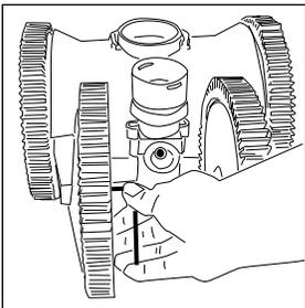
Once off, fold the tire off the Wheel Hub (step 3 above). To replace stretch the tire over the Wheel Hub (starting from one side and folding it back on). Make sure the tire is on correctly.
