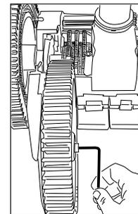
**6** Place the Shroud back onto the POOL-CLEANER™ making sure it's on correctly. Drop the three screws into the screw holes and secure.
