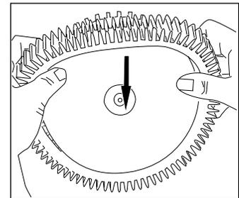
**4** **TO REMOVE THE 4X POOLCLEANER™ BACK TIRES** you will need to remove the Shroud with a Phillips screwdriver (see pg. 11 step 3) and then remove the Wheel Hubs with a 5/32" or 4 mm Allen wrench turning the wrench counterclockwise.
