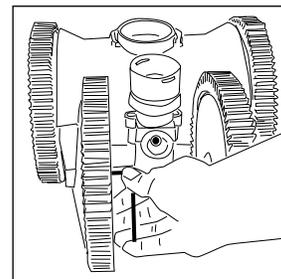
**6** Rotate the right front tire forward to ensure that it moves smoothly. If not you fastened the wheel hub incorrectly.
