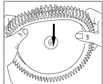
**4** **BACK TIRES** remove the Wheel Hubs with a 5/32" or 4mm allen wrench turning the wrench counterclockwise.
