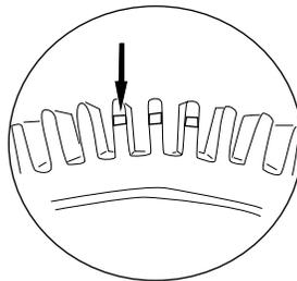
**3** Place the cleaner on a work surface. **TO REMOVE THE POOL-CLEANER™ FRONT TIRES**, use only your hands (other objects may damage the POOLCLEANER™) simply fold the tire off from top to bottom.
