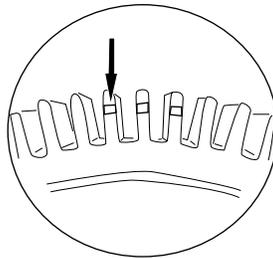
**3** Place the cleaner on a work surface. **TO REMOVE THE 2X POOLCLEANER™ TIRES OR 4X POOLCLEANER™ FRONT TIRES**, using only your hands (other objects may damage the POOLCLEANER™) simply fold the tire off from top to bottom.
